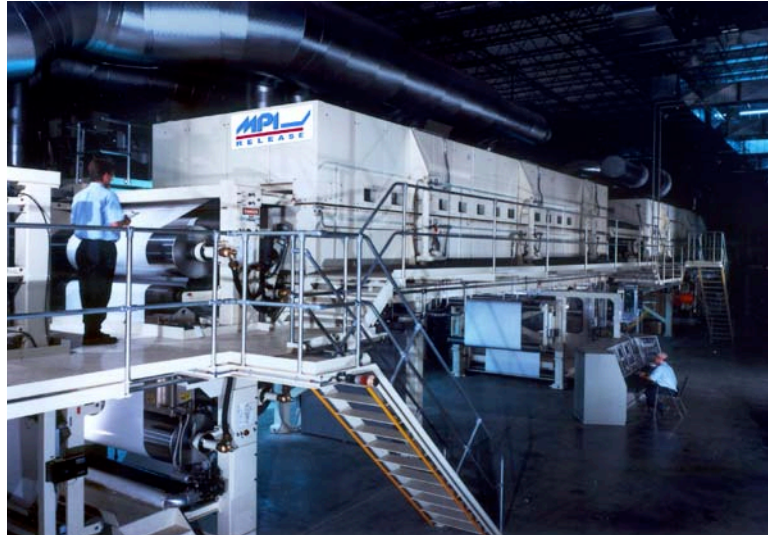
MPI's High-Speed Polytype Thermal Coater with inline printing capabilities.
