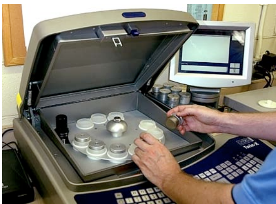
An Oxford Analyzer used to measure coat weight – part of MPI's extensive testing and research capabilities.
