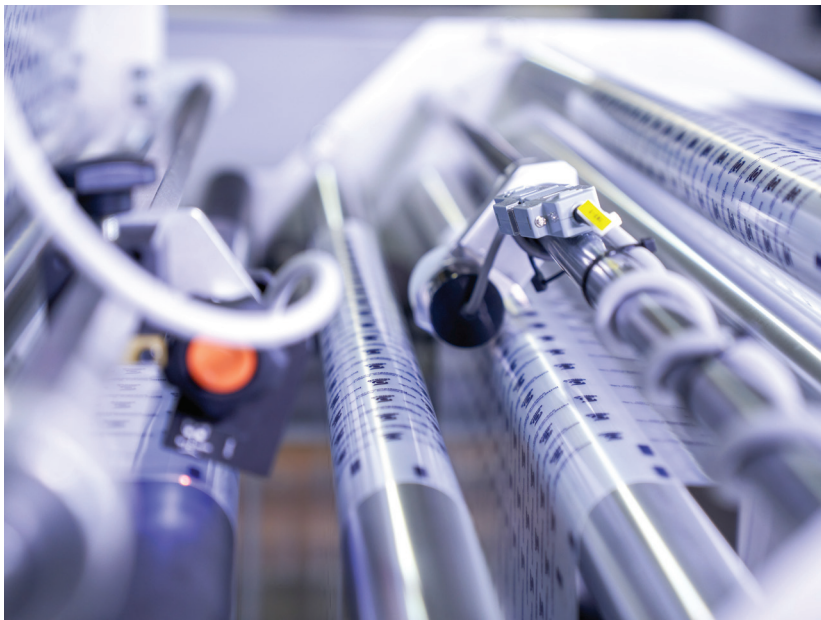
The main unwind has an encoder for tension control and an edge guide to ensure proper film position.
