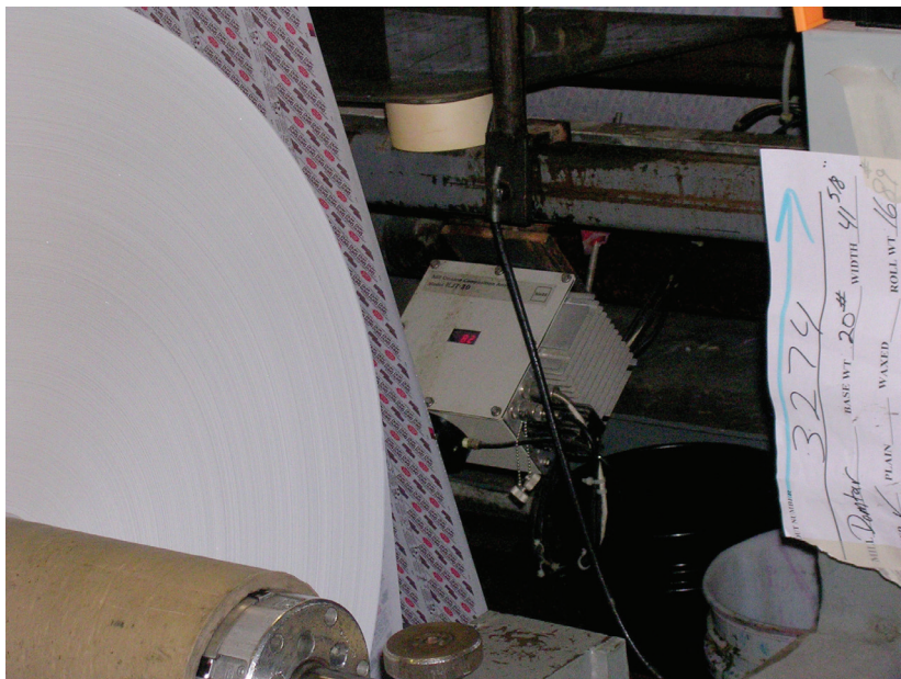
The size of a camcorder, the unit is designed for frequent spot checks wherever necessary, on both stationary and moving (process line) products.
