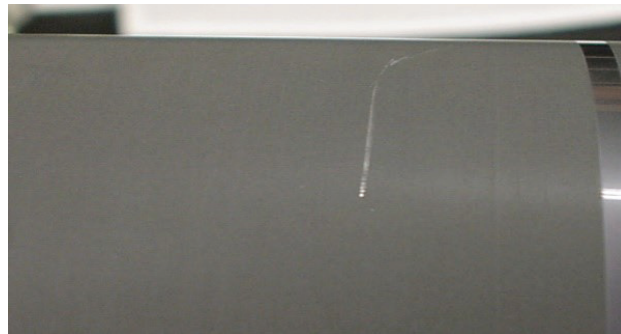
Anilox damage from something brushing up against it.
