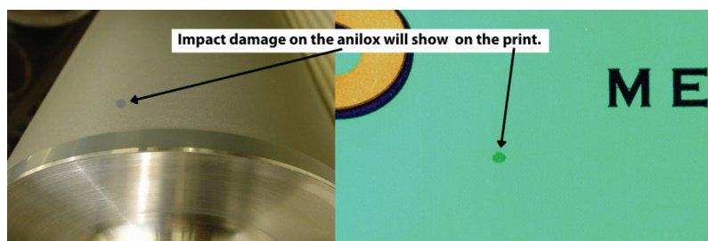
Impact damage on the anilox will show on the print.
